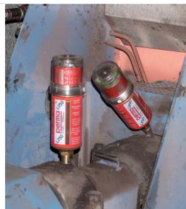
Lubrication system: 2 x perma STAR VARIO 250 cm 3
