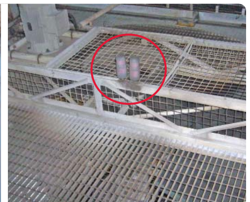
Lubrication system: 2 x perma STAR VARIO 120 cm 3
