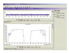
The system has been proven to provide advance warning of faults with both rolling element and plain bearings, balance and clearance problems. This greatly helps reduce the number of major failures and allows accurate maintenance planning.
